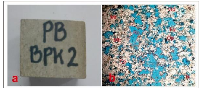
Figure 3. a). Fine calcarenite sample with negligible porosity using the density analysis method b). Negligible porosity using the petrographic observation method (PPL)
