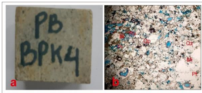
Figure 5. a). Medium calcarenite sample with negligible porosity using the density analysis method b). Negligible porosity using the petrographic observation method (PPL)
