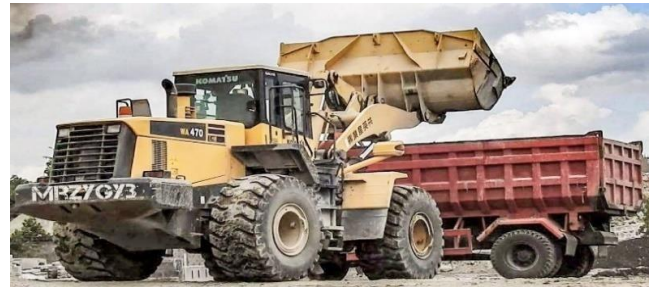
Gambar 1. Whell Loader Loading ke Dump Truck
